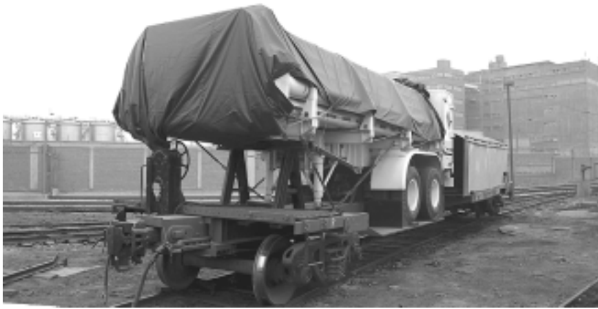
> The railway employed a borrowed CNG highway tanker mounted on a modified flatcar to act as locomotive tender during the tests, so as to evaluate ECI's Economizer dual fuel system.
