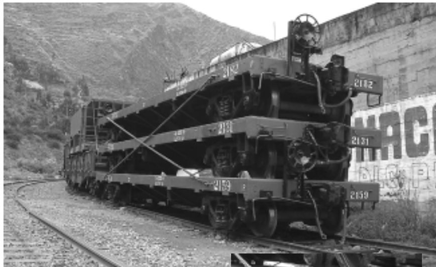
> From an operational point of view, triple stacking of flatcars will lower the quantity of trains the railway needs to run upgrade for the repositioning of empties. The modifications needed to stack the cars are quite simple and straightforward.
