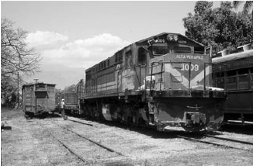
> FVG's No. 1009, Bombardier/Alco Co-Co 2000 HP "Alta Verapaz", at the head end of a freight train loaded with steel products. The powerful MX 620 locos are used on the relatively flat section of the railway between Puerto Barrios and El Rancho. Their long three-axle trucks are not flexible enough to enable them to perform reliably on the winding and steeply graded sections of the line (Frank Stenvall).
